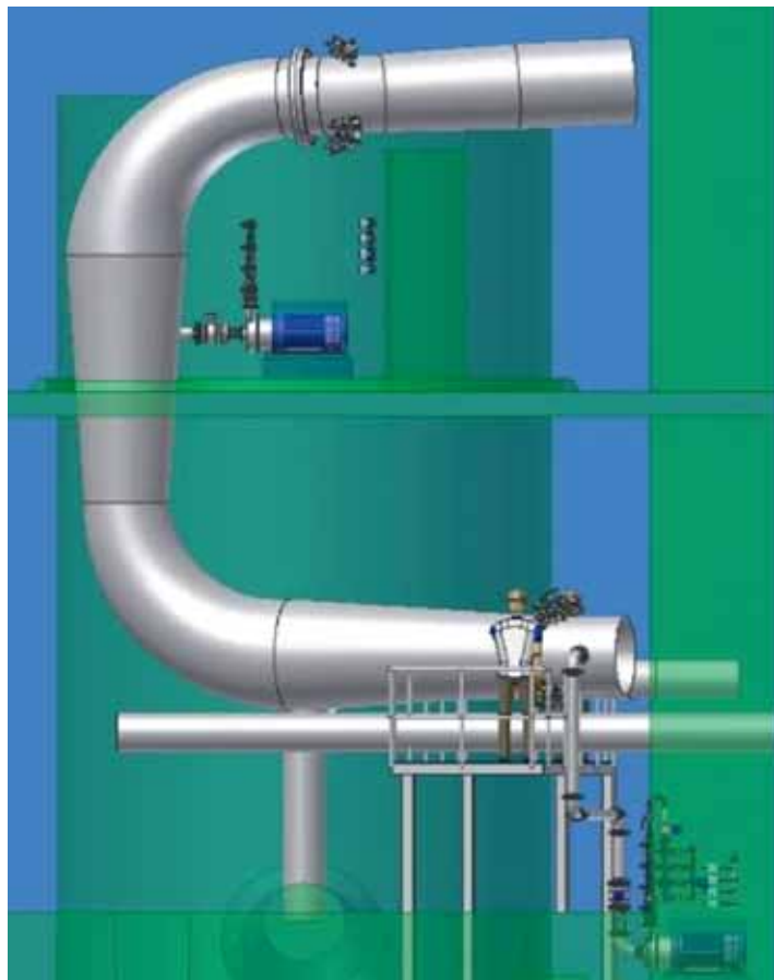
Above: Newsprint & directory paper production line: Two TrumpJet mixing stations installed on the 800 mm process pipe between the screen and head box.
