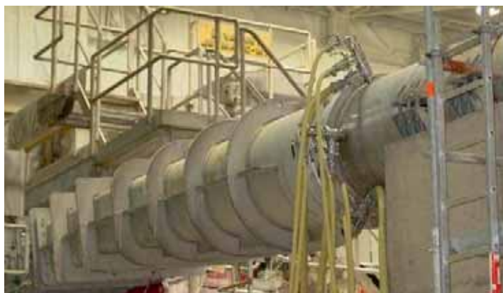
Above: Newsprint & directory paper production line: Two TrumpJet mixing stations installed on the 800 mm process pipe between the screen and head box.
