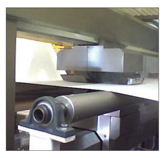
Scienta has pioneered the use of processor controlled measuring heads capable of real-time linearisation of the measurement signal. Thanks to Fieldbus connection the output signal can be easily and accurately interfaced to all sorts of computer and PLC equipment.
