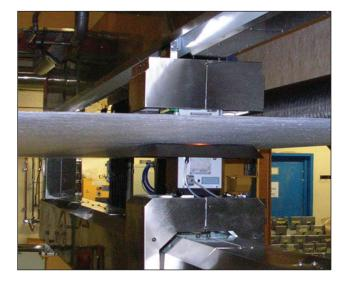
**NIR moisture meters** are highly accurate due to 'same spot' measurement. It is maintained even with very low moisture content. As with all Scienta Sensors, the NIR measuring head is intelligent. The integrated processor handles linearisation, calibration and communications tasks. Stand-alone sensors are easy to interface directly to an Operator Panel using standard interfaces.
