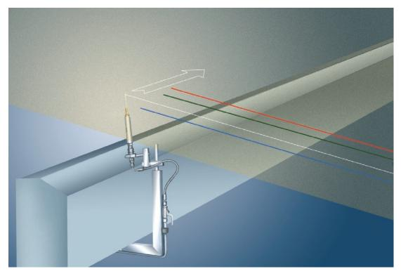
With a press of a button, the cutting head moves to the desired, pre-programmed tail width. Output signals of the cutting head positions can be used in process control.
