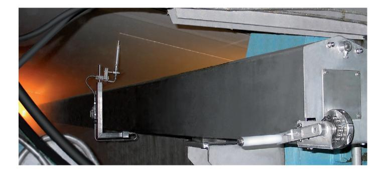
Successful tail feeding is based on accurately controlled tail cutting. Fastpap WetCut is a wet-end tail cutter which represents the greatest expertise in its field. With a press of a button it moves to a pre-programmed tail width and, after threading, it quickly widens the web.
