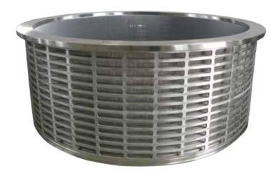
Johnson Screens' caged screens are designed to work in harsh environments. These screens use a reinforced stainless steel cage and are designed to give more rigidity and strength than other designs. Using a steel webbed structure, creates force multiplying strength to the rings and a stiffeners to reduce moments of inertia. With this design, Johnson Screens' caged screens distribute the pressure drops over a larger area of the structure increasing life and longevity.
