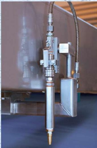
Fastpap WetCut is easy to install into existing process. Depending on the location, it can be installed either on top of or below the paper web.
