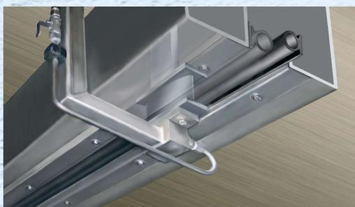
All moving parts are inside the beam, which is well sealed to keep the components clean
