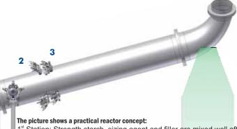
1<sup>st</sup> Station: Strength starch, sizing agent and filler are mixed well after the headbox screen,
