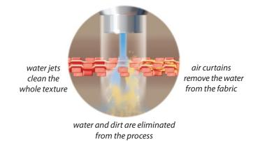
The save-all is located under the fabric, so no paper broke can get jammed in it, and this is also the most effective direction for removal of the impurities. Since the fabric is not cleaned against the roll, the impurities do not get into the inner cycle or stick to the roll surface.
