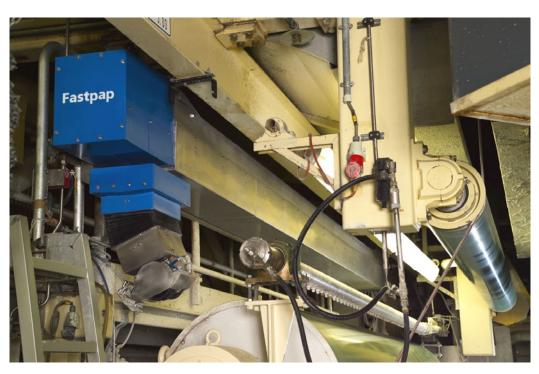
Fastpap LineSprint installed at a coating station for cleaning of the backing roll.
