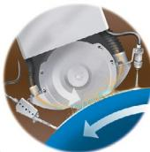
It is possible to clean the whole width of the roll or only a certain part of it. All impurities detached from the roll surface, and any water used while cleaning, are vacuumed up and removed from the process. Efficient air doctors ensure surface dryness.
