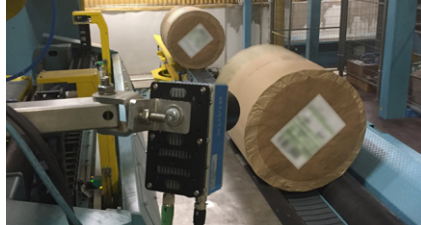
Roll Header and Label Analysis Roll header and label checking, analysis of bar codes and numbers. An alarm for critical faults triggered.
